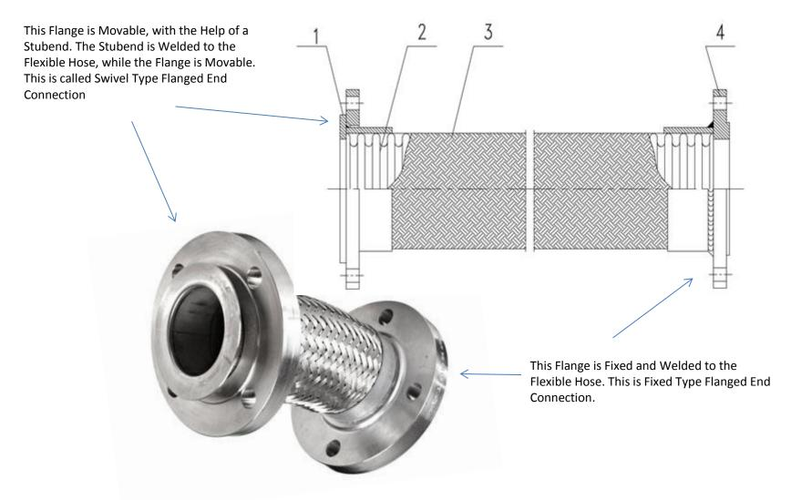
Types of Flanged End Flexible Hoses: Both Side Fixed, Both Side Swivel Type or One Side Fixed & One Side Swivel
